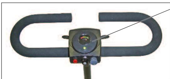
On/off switch, speed control and paddle controls, forward/reverse
