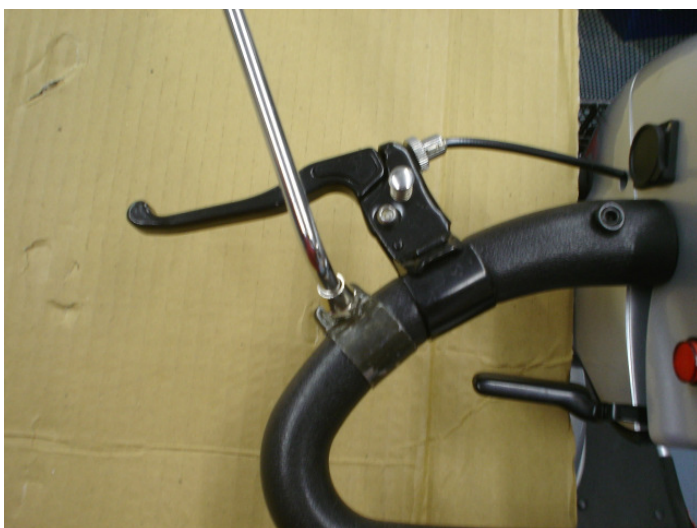
Remove the brake cable and handle.
