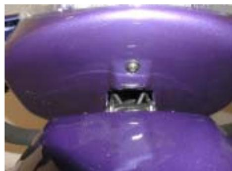
3. Remove the headlight when it has been angled from bottom to top.
