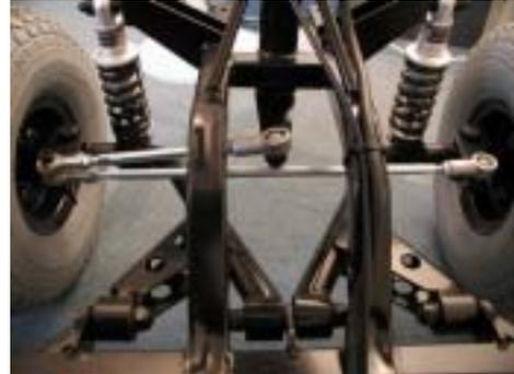
2. Screw the stop, washer and nut to the Allen screw below the stub axle.
